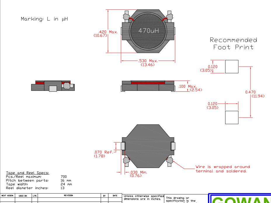
property of Gowanda Electronics. Copies shall not be reproduced or in. (mm) Part #: **SMP3308LP-Dimensional Specification** copied or used as the basis for the manufacture **ONE MAGNETICS PARKWAY** DRAWN APPROVED or sale of apparatus ΚВ ΚB ВМ GG without permission.
